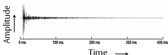
Fig 4. RIR recorded in a real seminar-room with a distance of 2.50 m between source and listener, giving a ratio of early (50 ms) to late energy of 9.71 dB (C50, left ear, A-weighted). Recorded using Farina’s swept-sine method (2000).
