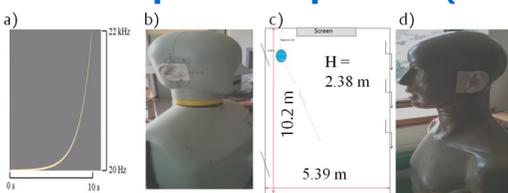
Fig 3a) Swept-sine measurement signal; b) played through KEMAR dummy with directional transducer mouthpiece; c) in real room; d) recorded at head-and-torso-simulator with mikes in ears; When RIRs are convolved with a sound and played over headphones, a listener should experience the sound as if heard in the original room.
