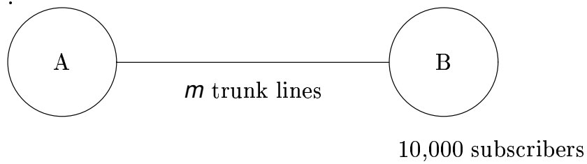
Figure 9.5: The telephone exchange.
