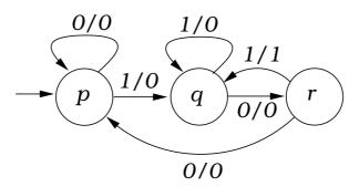
having been received or the last pair of characters received having been 00; q corresponds to the last character received having been a 1 and r corresponds to the last pair of characters received having been 10. The '1' arrow out of r is therefore labelled as giving output 1, indicating that a 101 string has been discovered.
