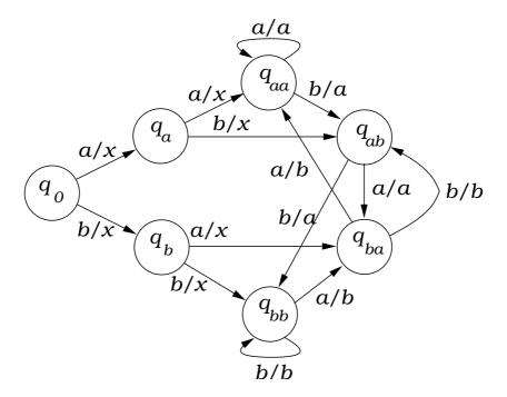
The starting state  $q_0$  corresponds to no input received so far. States  $q_a$ ,  $q_b$  correspond to only a single character, a or b having been received. States  $q_{aa}$ ,  $q_{ab}$ ,  $q_{ba}$ ,  $q_{bb}$  correspond to at least two characters having been received and the last two characters having been aa, ab, ba, bb, respectively. Given these interpretations of the states, the transition and output functions are obvious.
