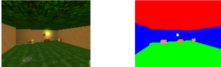
Fig. 1. On the left is the actual world rendered from the character's point of view. On the right, the world is rendered as using the synthetic vision module from the same point of view. Pink is used for a health power-up, orange for an ammunition power-up, yellow for a flying ball, green for the floor; blue for the wall and red for the ceiling.
