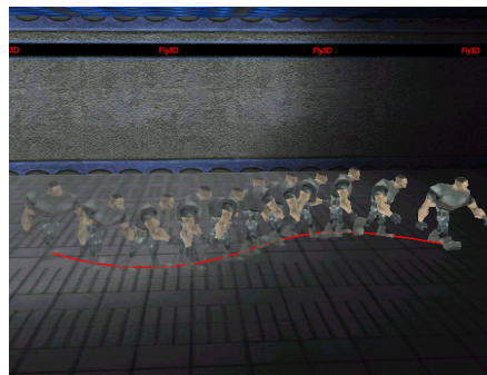
Fig. 3. a) Construction of a Bezier path; b) Bezier paths and obstacle avoidance; c) A character walking along a Bezier curve
