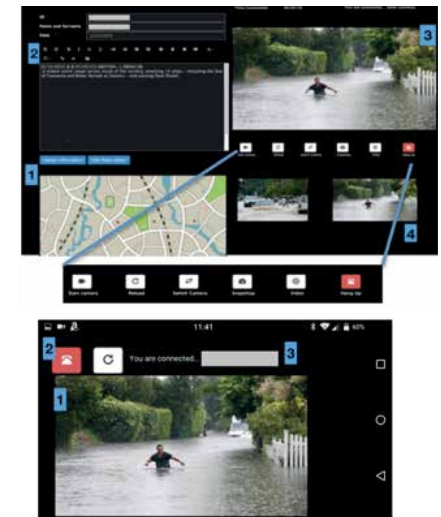
▲ Figure 4. Top - Eyes on the Ground control room (1 - geolocation of citizen, 2 - notes taken during video conversation, 3 - video stream from citizen's camera, 4 - media recorded during conversation). Bottom - Citizen camera view (1 - view of the content being streamed, 2 - call connection controls, 3 - a live text messaging area for detailed instructions).
