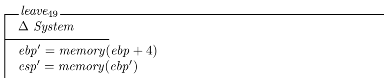
Figure 3.4: A simple specification for an instance of the x86 leave instruction
