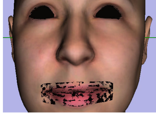
Figure 3.27: The hidden vertices project to the same depth and therefore fight to co-exist with the occluding vertices
