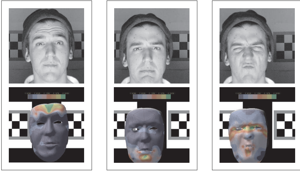
Fig. 5.11: Strain diagrams showing the modulus of compression, computed as the determinant of the tensor field \bar{S} defined over the fitted mask. This happens to be a measurement of local area reduction (see Section 5.2.1), arising with more intensity in the areas coded with colours to the right of the inset bar (down to 1/4 of the original area). Directions of maximum compression are oriented perpendicularly to the isocurves of such a scalar field.
